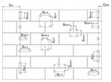
$\begin{array}{lll} C_{cr} & = & Characteristic \ edge \ distance \\ C_{min} & = & Minimum \ Edge \ distance \\ S_{cr} & = & Characteristic \ spacing \\ S_{min} & = & Minimum \ spacing \end{array}$
